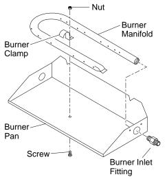
Figure 9 - Installing Burner
